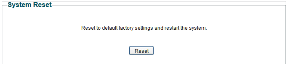
Figure 7-1 Resetting the Switch
